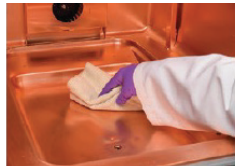
Figure 2: With shelves and cover removed, the integrated water reservoir is completely accessible for easy cleaning.
