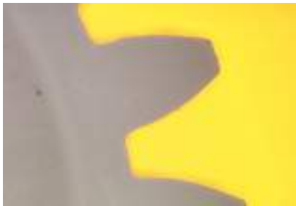
Plastic Gear Teeth with Smaller Module
