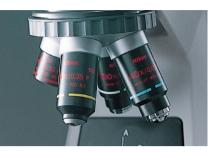
distances and higher N.A.'s to deliver startlingly clear images at any magnification because chromatic aberrations are corrected over the entire field of view. Nikon CFI optics employ an eco-glass that is manufactured with no harmful substances such as lead and arsenic.
