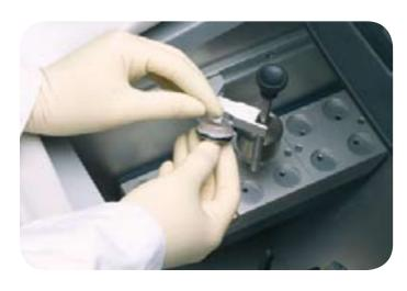
Cryomolds® provide a standardised, flat-surface with precise orientation to speed up sectioning.
