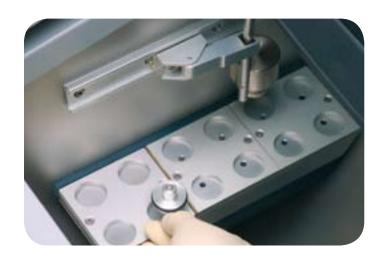
Position specimen on Cryobar<sup>®</sup>. For rapid cooling down to -50°C, place specimens on the Cryo+<sup>®</sup> portion of the Cryobar<sup>®</sup>.
