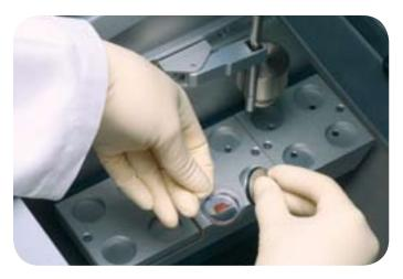
Easily orient specimen with Tissue-Tek® O.C.T.™ Compound using the Cryomold® technique. The heat extractor can be used to enhance freezing.
